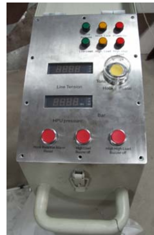
Remote Control Panel with Load Tension Meter
